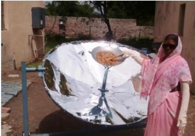
Giving a new dimension to concentrated solar system Leverage Net Solutions Pvt. Ltd. have commissioned a Concentrating solar dish Veggie dryer at Alpine Fruit Processing Pvt. Ltd. near Pune that also serves the purpose of cooking when situation demands. Realizing the might of a solar thermal system they decided to use the concentrating solar technology to accelerate drying process to that maximum moisture is removed from veggies and gives them a better rate to the dried veggies.
