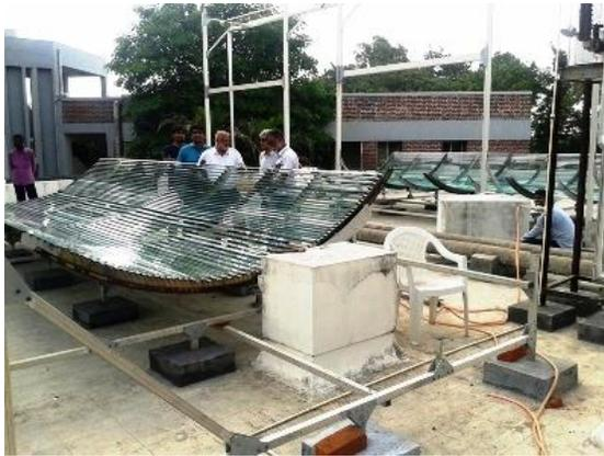
EnerSun Power tech Pvt. Ltd., Mumbai through and with help of Prof. Joshi and Prof Panse from ICT (Institute of Chemical Technology), Mumbai have indigenously developed a unique Concentrator Linear Fresnel Reflector (CLFR) to overcome the problems faced by parabolic dish concentrators and parabolic trough concentrators.
