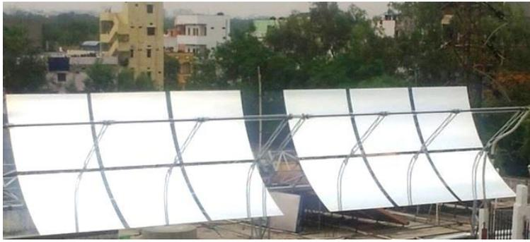
*Photo: Parabolic trough cooking system, courtesy: Oorja Energy Systems*
