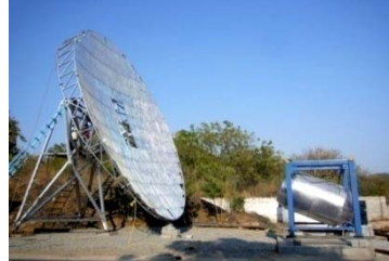
Fig. 5: Dual axis tracked Scheffler dishes with heat storage
